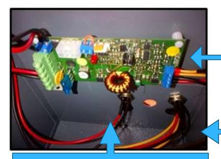
Open circuit protection without battery or load. When a PV panel is fully operational and in full sunlight, and plugged into the unit, without a battery or a load connected to it, the unit is not damaged, even if this condition continues permanently. It can withstand severe heat of up to 100 degrees C
