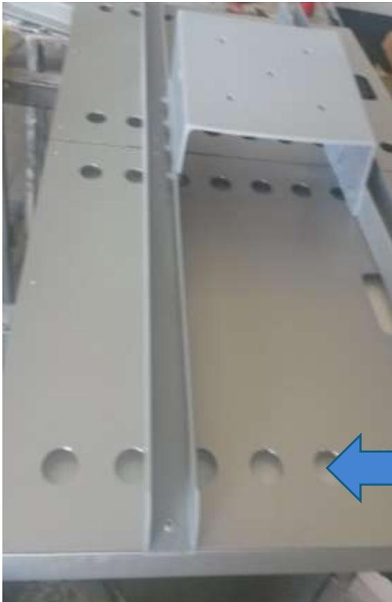
Connection between pole and solar panel ; it can rotate 360 degrees
