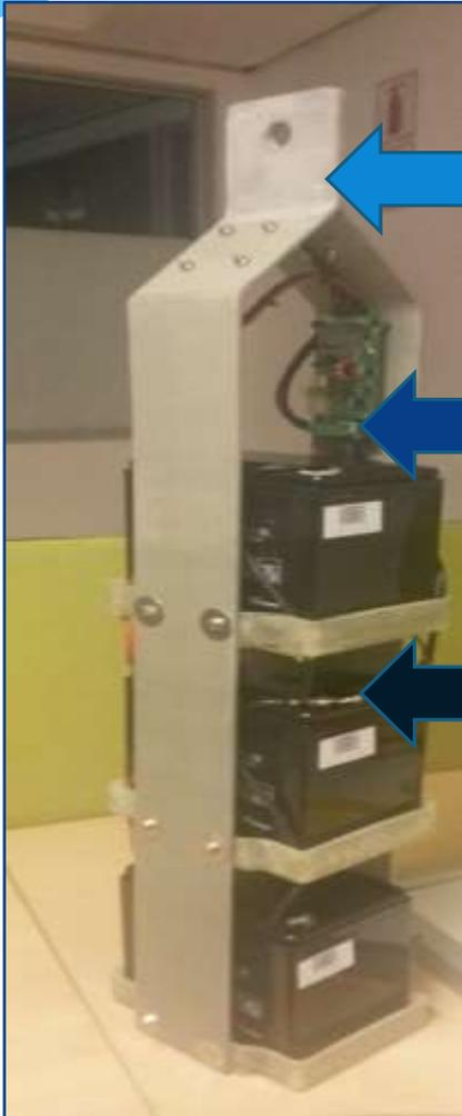
Fibre glass constructed battery housing structure dumped 1.5m below the ground
